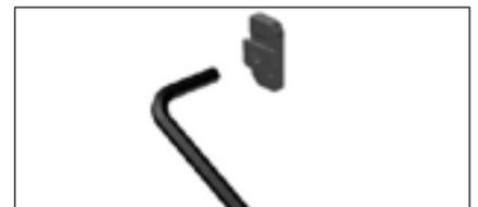
Position the Quarter Turn Buttons (C117) vertically into the gap between the Window and the Wallplate (A119 or A125) approximately 50mm in from the top and bottom of Window. Using the 6mm Allen Key, turn the button clockwise to lock them into position.
